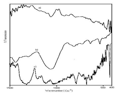
**Figure 5.** Infrared spectra for (a) polypyrrole, (b) sample B prepared from B solution that contains 0.01 mol pyrrole, 0.01 mol thiophene and 0.02 mol HBF<sub>4</sub>, (c) polythiophene prepared electrochemically.
