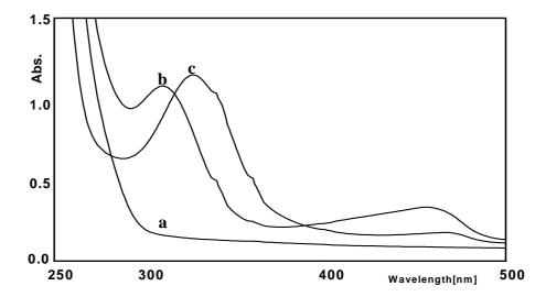
**Figure 1.** UV-vis spectra of (a) thiophene-HBF<sub>4</sub> mixture (1:1), (b) pyrrole-HBF<sub>4</sub> mixture (1:1), (c) thiophene-pyrrole-HBF<sub>4</sub> mixture (1:1:2), (The concentrations of species, C = 0.001M).
