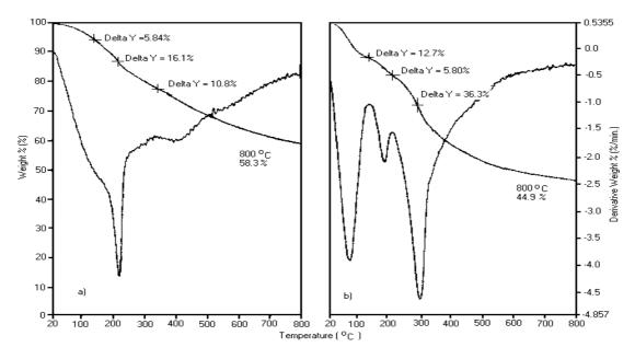
**Figure 3.** TGA curves for (a) polypyrrole homopolymer, (b) sample B prepared from B solution that contains 0.01 mol pyrrole, 0.01 mol thiophene and 0.02 mol HBF<sub>4</sub>.
