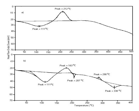
**Figure 4.** DSC curves for (a) polypyrrole homopolymer, (b) sample B prepared from B solution that contains 0.01 mol pyrrole, 0.01 mol thiophene and 0.02 mol HBF<sub>4</sub>.
